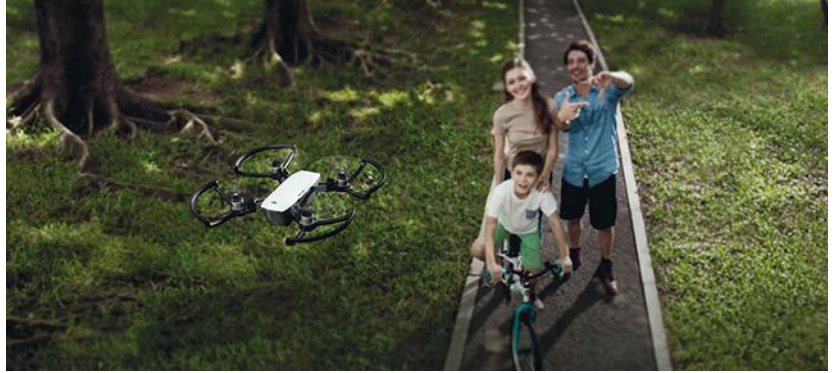
3. DJI's SPARK drone uses Intel's Myriad 2 visual processing unit (VPU) with ML support to recognize gestures such as framing and taking a picture.
